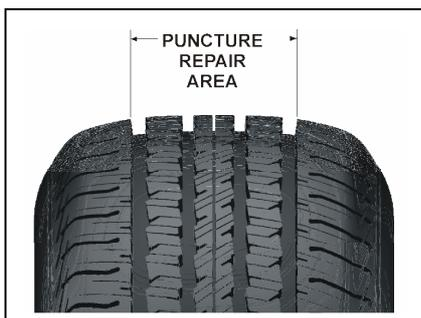
This graphic indicates that puncture repairs are limited to the tread area as generally depicted in the graphic.
